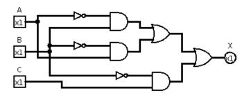
(h) Do the Quine-McCluskey procedure on the original circuit, show all steps in the derivation. Construct the minimized logical circuit function in SOP form. Solution:
