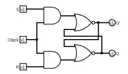
Using a clocked SR flip-flop, draw the diagram for a D flip-flop.
