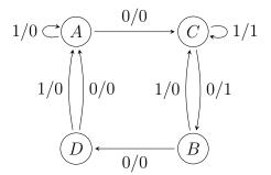
12. Design a sequential circuit that detects an input sequence of 1001 with overlap. Use only JK flip-flops in your construction.
