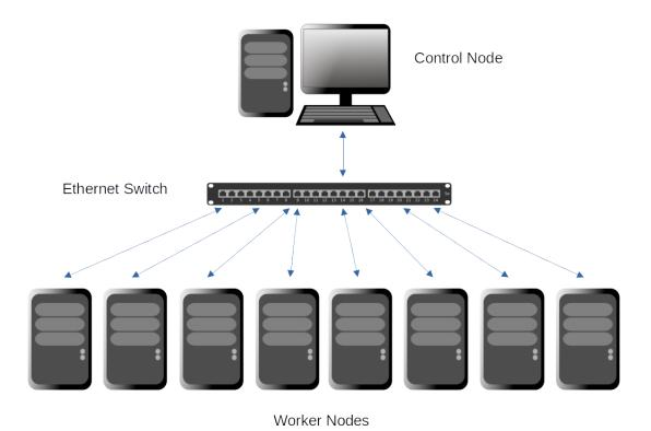
In a simple Beowulf cluster the only computer that has a monitor, keyboard, and mouse is the control node. All the worker nodes are simply the machine connected to the Ethernet switch. The control node will be able to access all the worker nodes, and use their hardware for computations, through ssh (Secure Shell) using the terminal.
