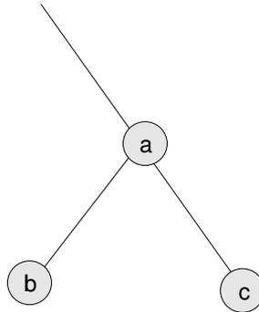
The new value is  $c$ . We can restore the heap property of this subtree by comparing  $c$  to  $a$ . If  $c$  is smaller, then the heap property is satisfied. If  $c$  is larger, then we swap  $c$  and  $a$ . The swap satisfies the heap property because we know that  $c$  must also be bigger than  $b$ , because  $c > a$  and  $a > b$ .
