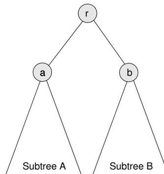
The root node has priority `r` and two subtrees, A and B. The value at the root of Subtree A is `a` and the value at the root of Subtree B is `b`.
