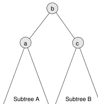
Again,  $c$  is the value we copied from the last element in the array and  $b$  is the highest value left in the heap. Since we haven't changed Subtree A at all, we know that it is still a heap. The only problem is that we don't know if Subtree B is a heap, since we just stuck a (probably low) value at its root.
