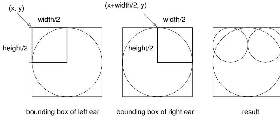
As shown in the figure, the coordinates of the upper-left corner of the bounding box for the left ear are  $(x, y)$ . The coordinates for the right ear are  $(x+width/2, y)$ . In both cases, the width and height of the ears are half the width and height of the original bounding box.
