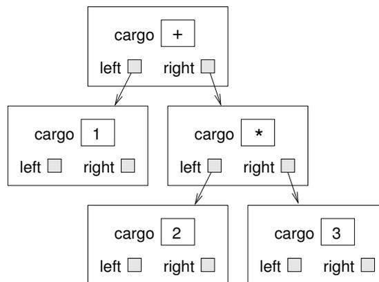
The nodes can be operands like 1 and 2 or operators like + and \*. Operands are leaf nodes; operator nodes contain references to their operands (all of these operators are **binary**, meaning they have exactly two operands).
