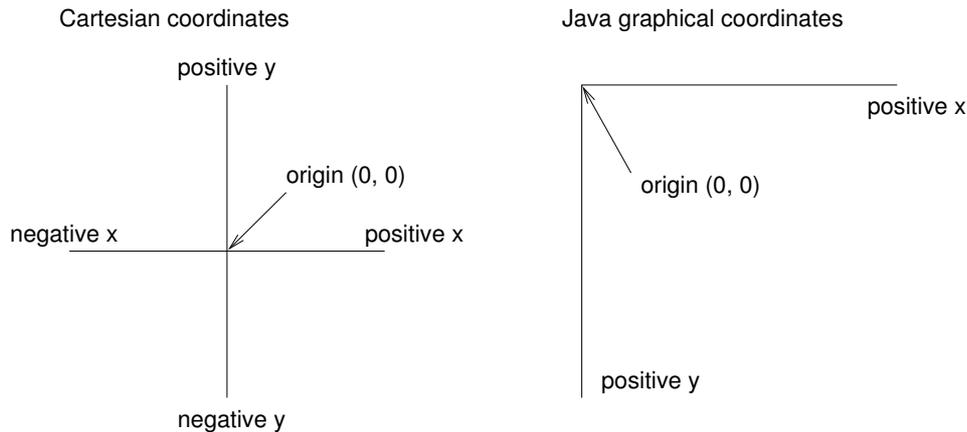
Annoyingly, it is conventional for computer graphics systems to use a variation on Cartesian coordinates in which the origin is in the upper-left corner of the screen or window, and the direction of the positive *y*-axis is *down*. Java follows this convention.
